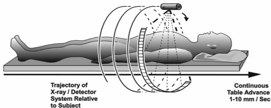
**Fig. (2.1):** Schematic of helical CT scanning (Erik L, 2006).
