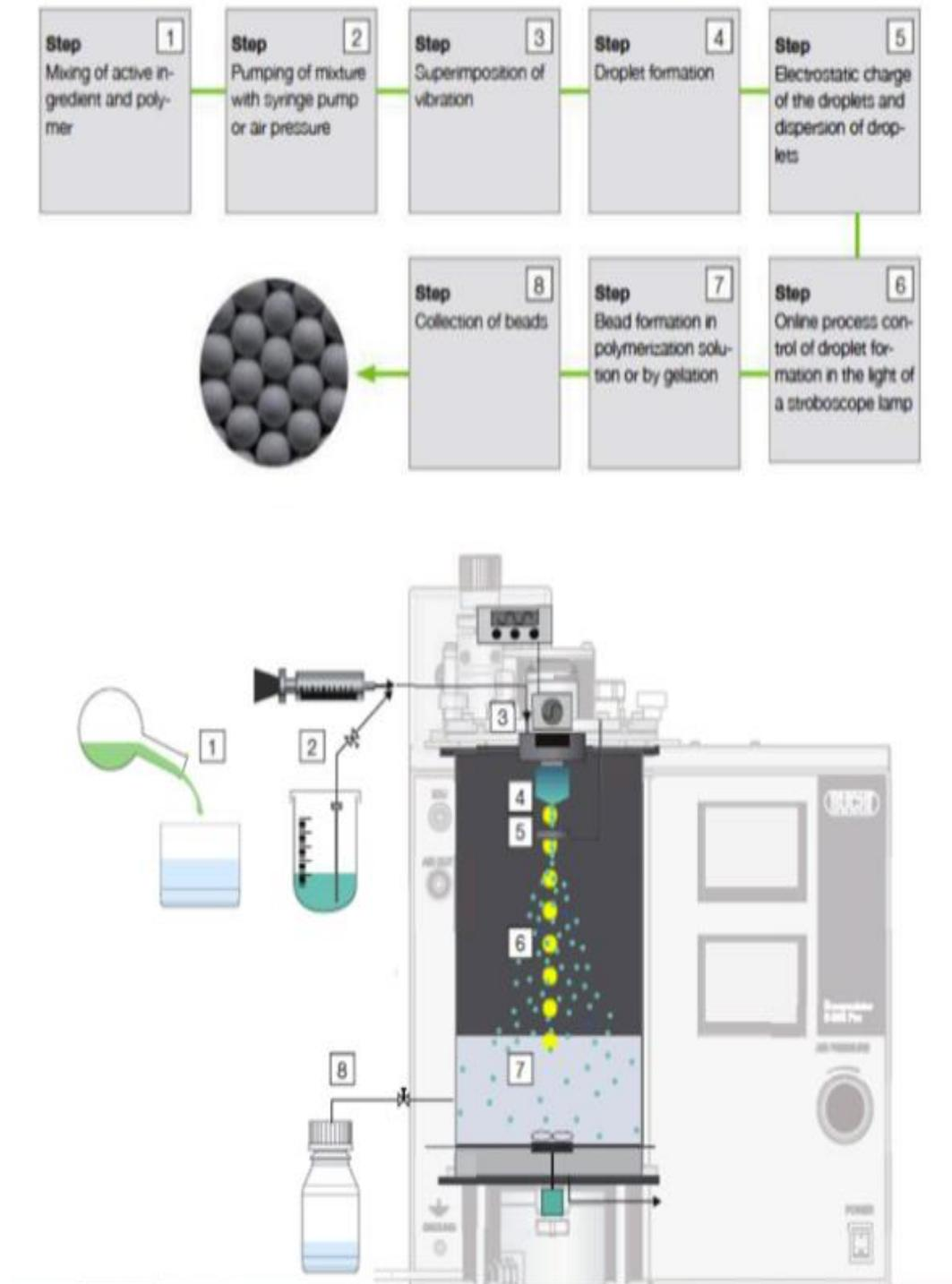
**Fig. 2.1** Functional principle of vibrating technology using BUCHI Encapsulator B-395 Pro (BUCHI; Switzerland; De Prisco *et al.*, 2015)
