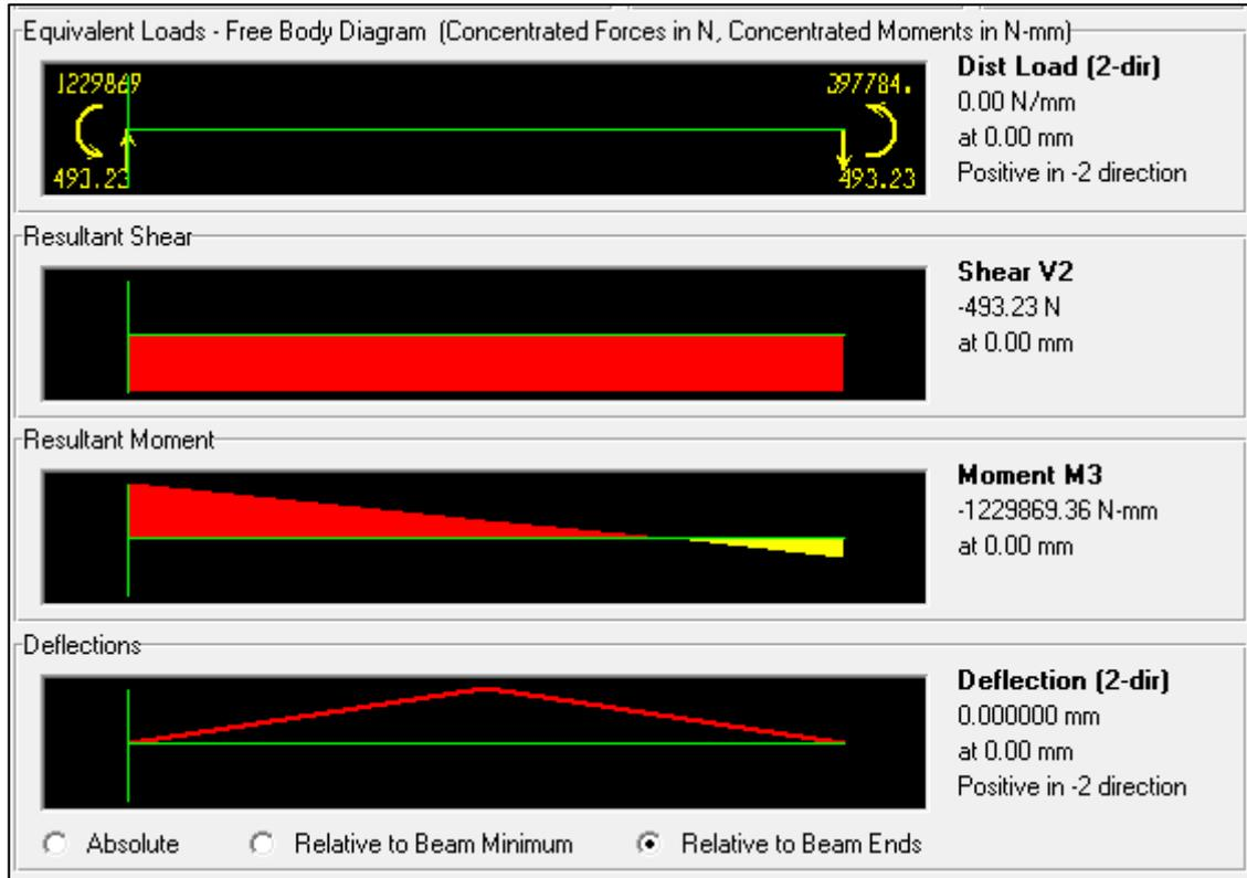
**Figure (4.19):** Virtual shear and moment diagrams for the left column in the bare frame of model (W5 C50) used for verification by the virtual work method, as obtained from SAP2000
