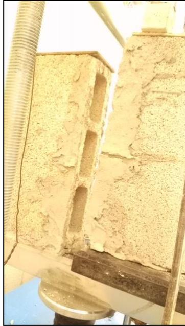
**Figure (3.9):** Failure of the specimen during the shear test
