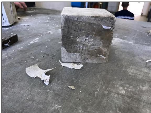
**Figure (3.2):** A mortar specimen used in the experimental test of this thesis
