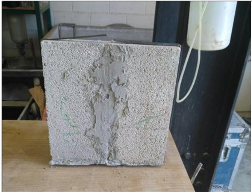
**Figure (3.3):** The connected bricks which were used for the shear test
