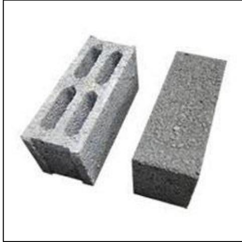
Figure (2.7): Hollow brick samples
