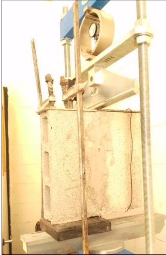
**Figure (3.5):** The shear test of a specimen of mortar-connected two bricks using the Tile Testing Machine
