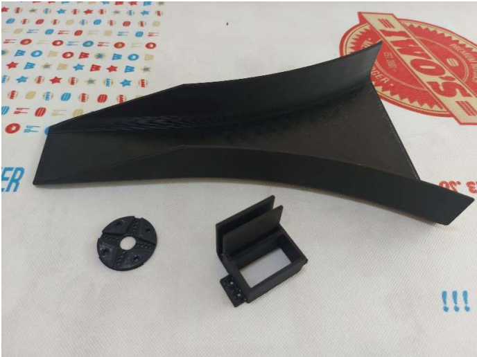
Figure (3.25): Bottle's slider.
