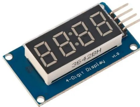
Figure 3.22: 4-digit 7-segment display for timing.
