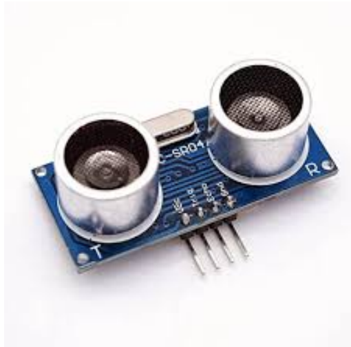
Figure 3.6: Ultrasonic sensors used for motion control.
