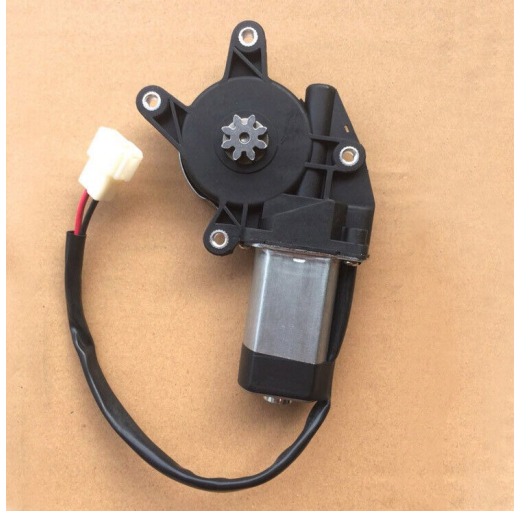
Figure 3.4: Window Motor used for movement.
