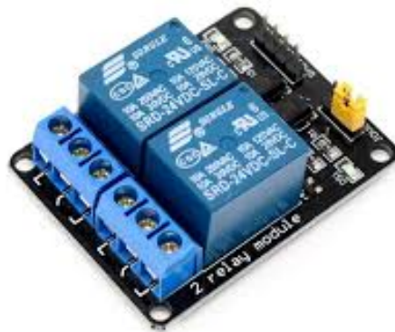
Figure 3.5: Two-channel Relay for controlling the motor.
