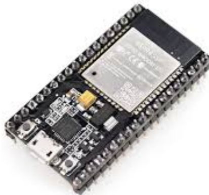
Figure 3.9: ESP32 used as WiFi access point for control.
