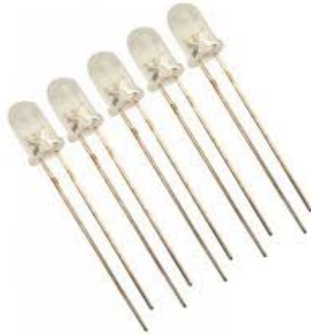
Figure 3.24: White LEDs for LDR detection feedback.
