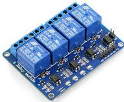
Figure 3.7: 4-Channel Relay for controlling lights.
