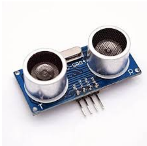
Figure 3.23: Ultrasonic sensor for sound frequency control.
