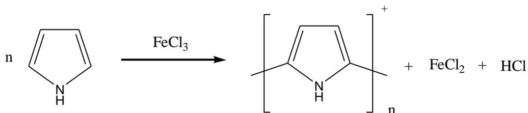
**Fig 1.4:** Chemical polymerization of polypyrrole
