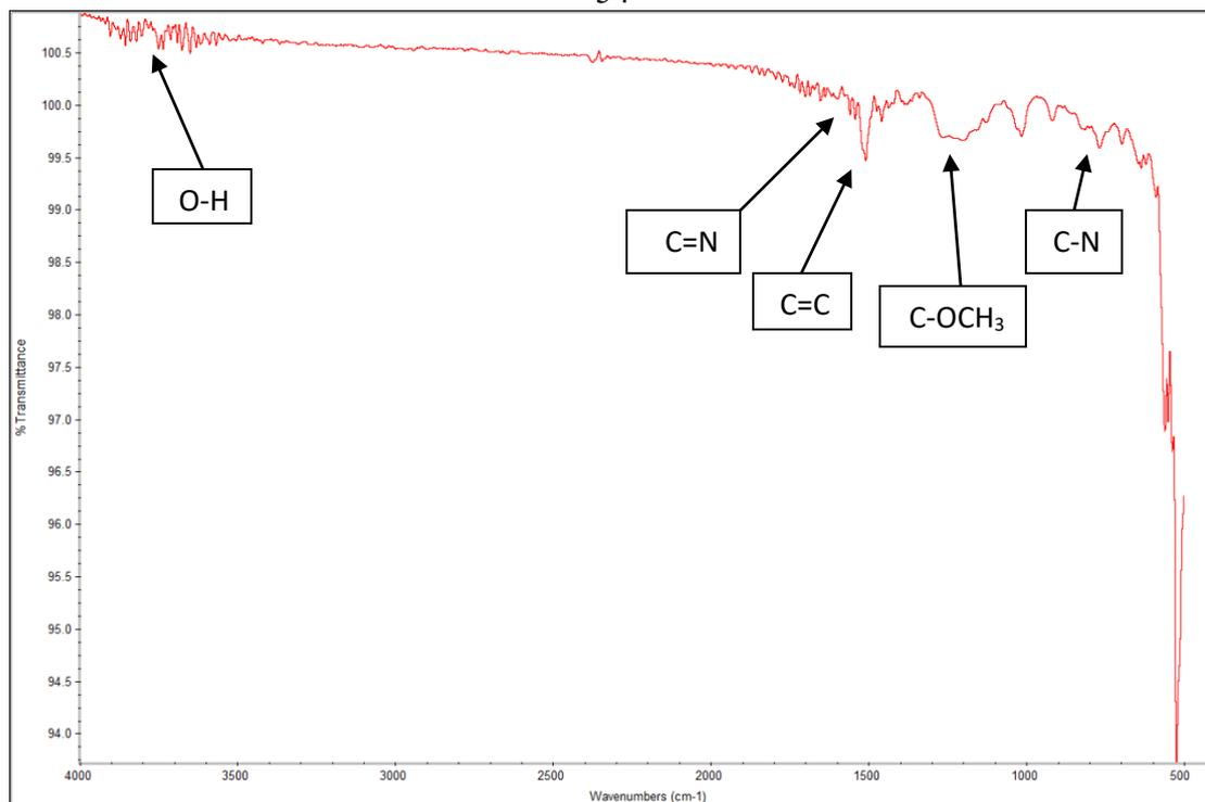
**Fig 3.14:** FT-IR spectrum of curcumin-pyrazol derivative (11).
