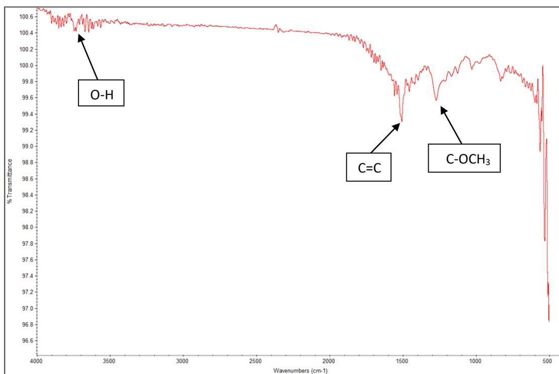
**Fig 3.19:** FT-IR of curcumin based polymer cross-linked with  $\text{Cu}(\text{CH}_3\text{COO})_2$  (13)
