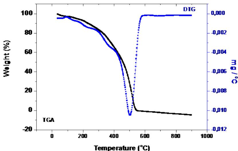
Fig 3.8: DTG thermogram of curcumin based polymer (5)
