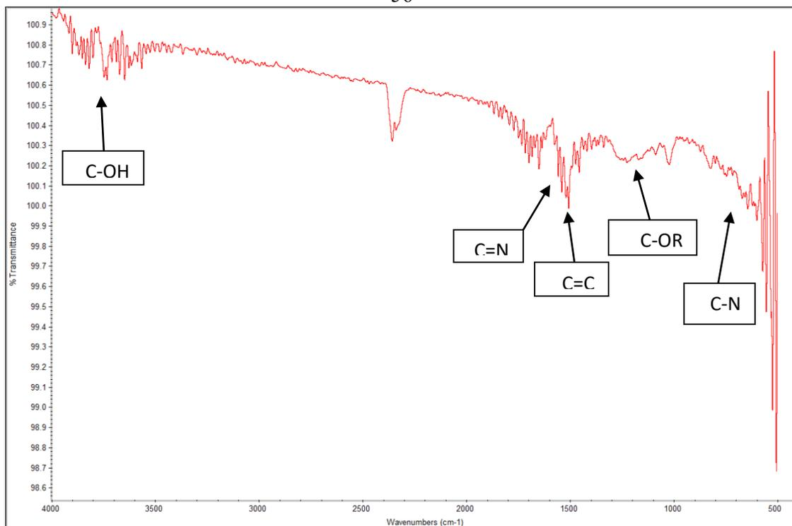
**Fig 3.16:** FT-IR spectrum of curcumin based polymer with pyrazole pendent group (12).
