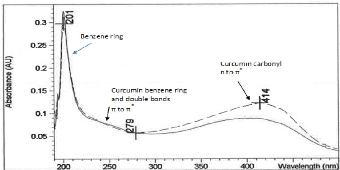
**Fig. 3.6:** UV spectrum of the polymer (5).
