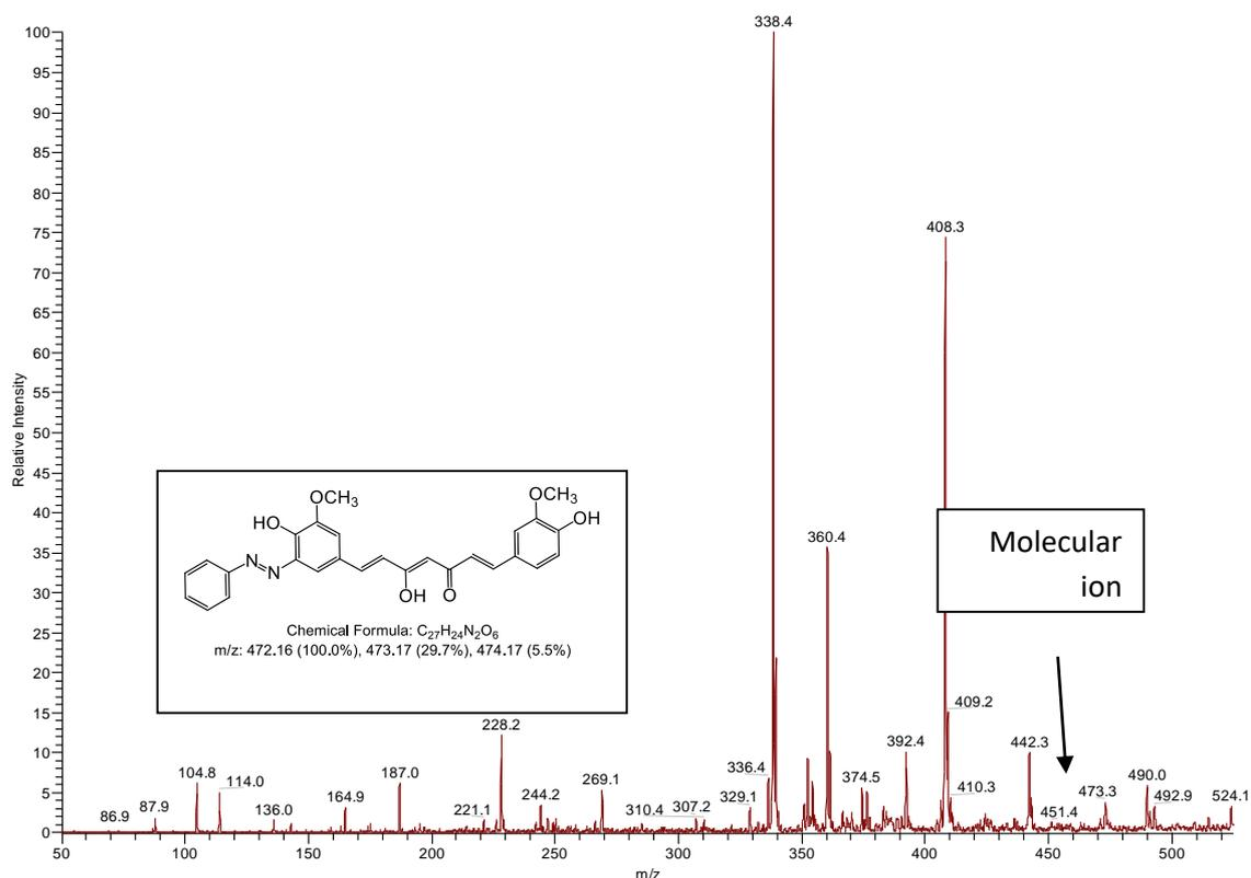
**Fig 3.5:** MS of polymer (5) shows the molar mass of the repeat unit
