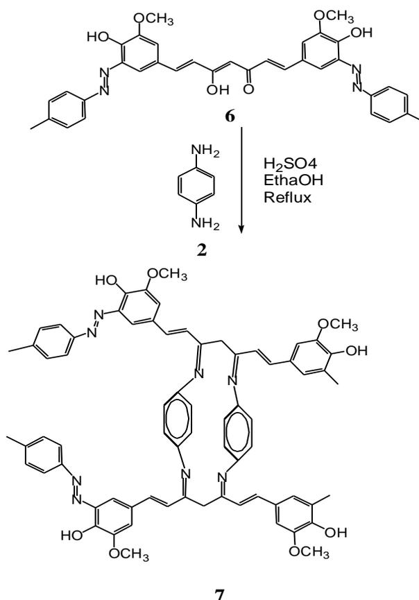
**Fig 3.10:** Preparation of cross-linked polymer
