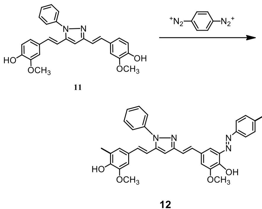
**Fig 3.15:** Synthesis of curcumin based polymer with pyrazole pendent group
