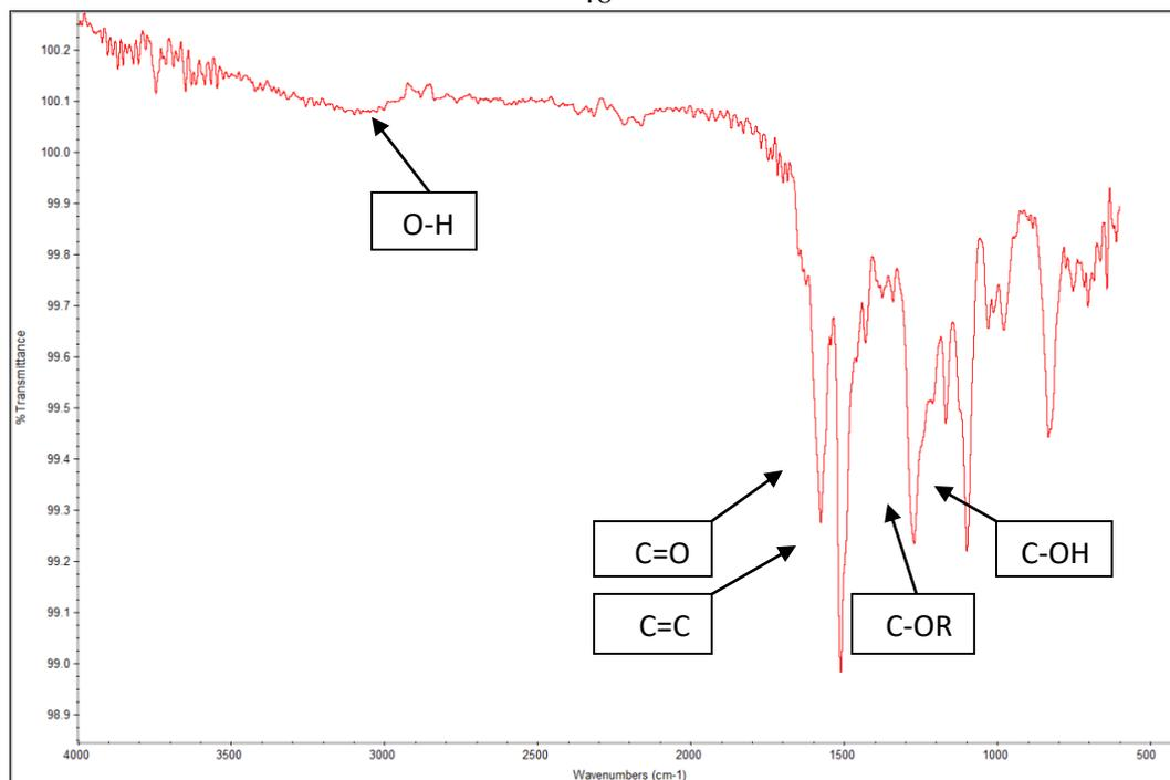
**Fig 3.7:** FT-IR of the curcumin based polymer (5)
