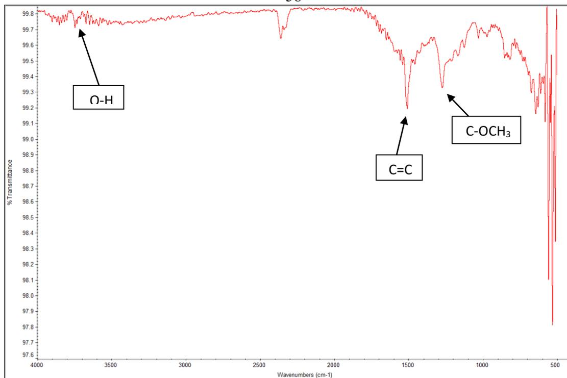
**Fig 3.18:** FT-IR of curcumin based polymer cross-linked with  $\text{FeCl}_2$  (14)
