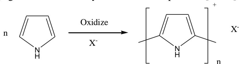
**Fig 1.3:** Electrochemical polymerization of polypyrrole
