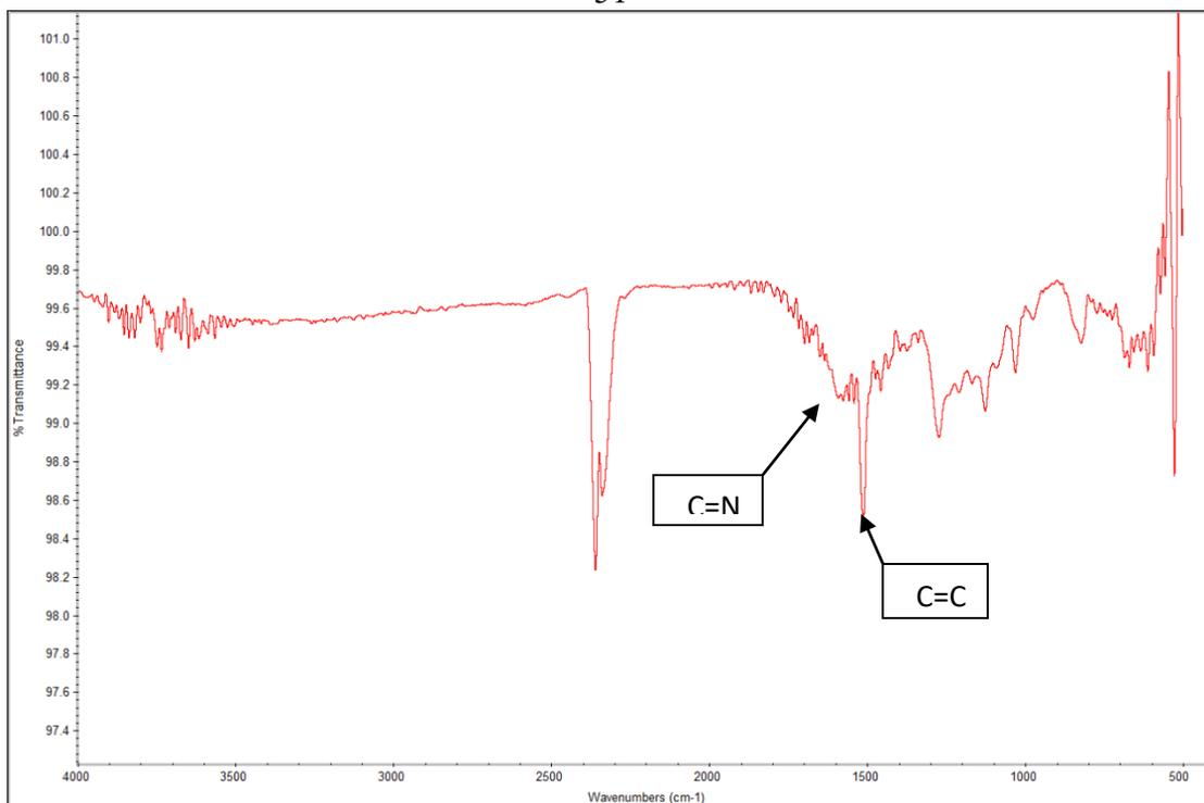
**Fig 3.11:** FT-IR of cross-linked polymer (7).
