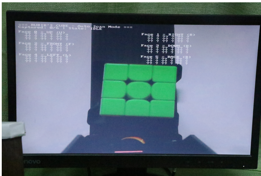
Figure 4.5: VGA hardware display showing real-time system status, scanning progress, and operational parameters.
