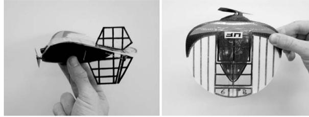
Figure 2.3: Micro air vehicle has a 150 (*mm*) wingspan and equipped with a video camera (Samardžić et al. 2014).
