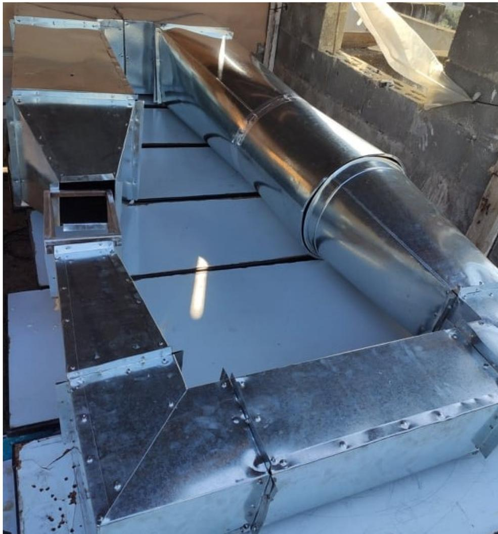
Figure 4.3: Final view of the scaled wind tunnel.
