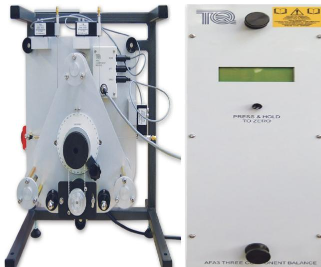
(a) Three-component balance. (b) Digital display.
