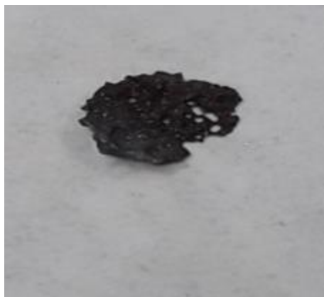
Figure 11: A copper coin after EDTA, acetic acid and hydrogen peroxide treatment; the material is entirely corroded
