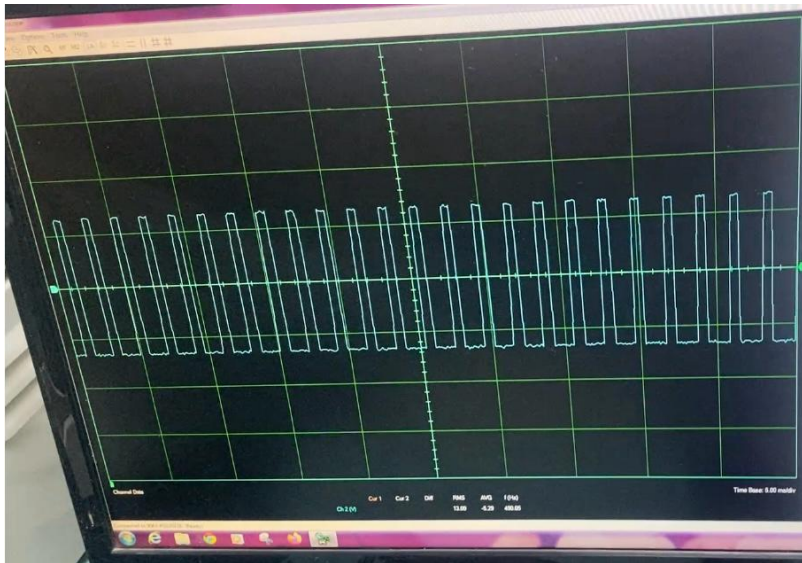
Fig. 6.3.1 PWM Output Signal from Arduino to L298N H-Bridge
