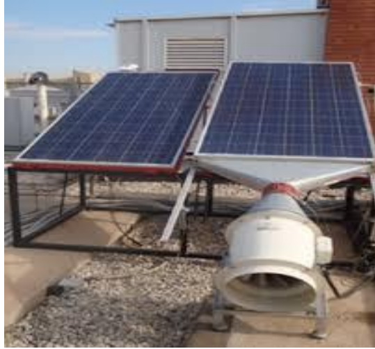
Figure 2: Hybrid solar Photovoltaic/Thermal system cooled by forced air circulation.
