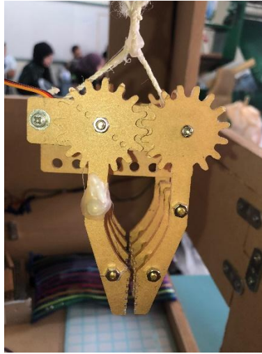
Figure 8 Custom Gripper 3D Printed Parts
