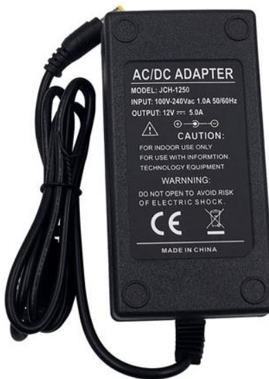
Fig19.Example for a Voltage Converter.
