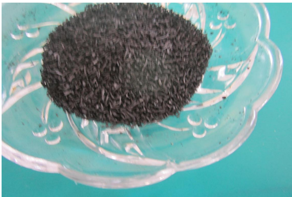
Figure 4.2: Magnified picture of cypress fruit activated carbon
