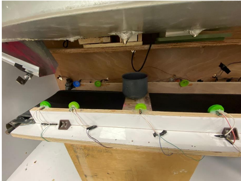
Figure 4.9 : bowl is moving to fill basic materials using car motor.
