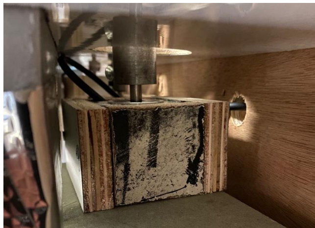
Figure 4.10 : NEMA23 stepper motor with couplers.
