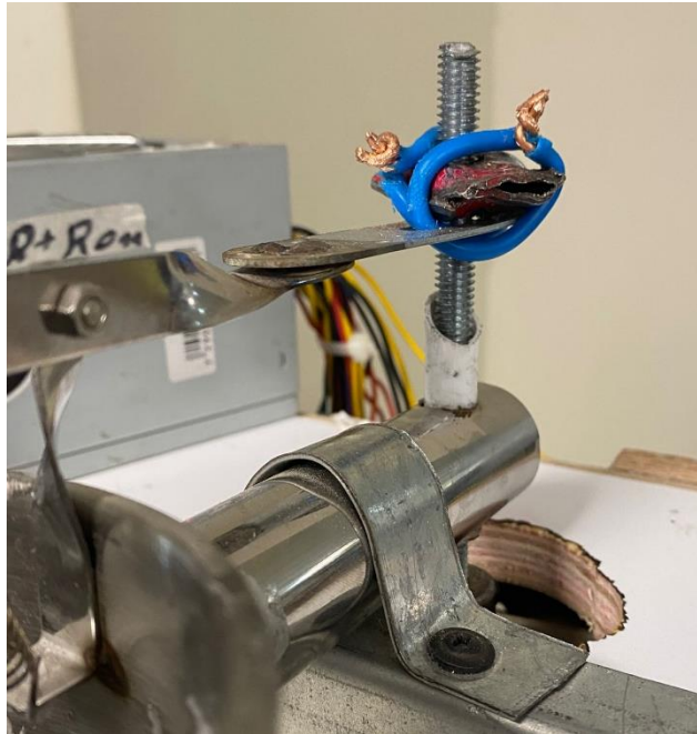
Figure 4.11 : Screw connecting the coupler to the outlet.
