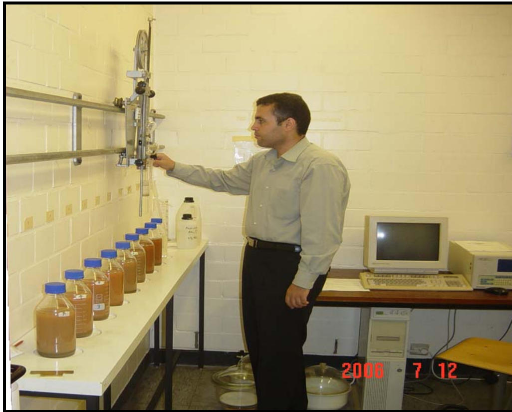
Figure (54): The Device and Bottles Used in Soil Texture Test.
