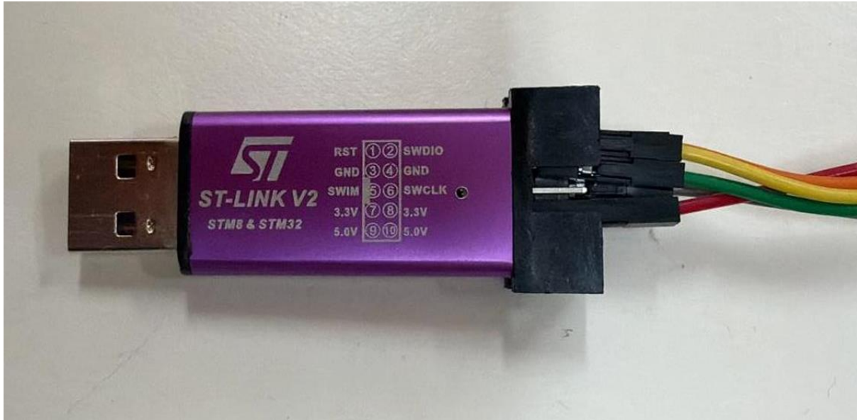
Figure 6.4: The ST-LINK/V2 debugger/programmer used for flashing the STM32 microcontroller.
