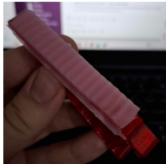
Figure 4.10: TPU Finger - Silicon Coated
