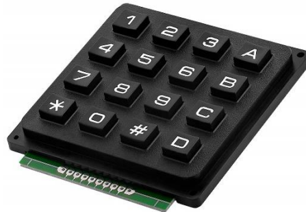
Figure 30 : 4x4 keypad for selecting pots and controlling system actions.
