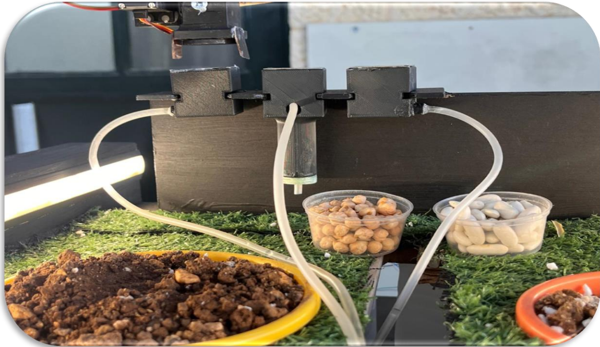
Figure 16 : Magnet-based tool heads allow automatic swapping for watering, fertilizing, and seed planting.
