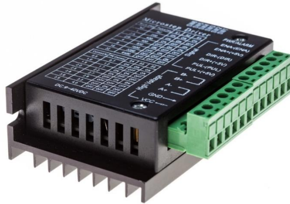
Figure 10 : 3.5 A stepper driver controlling the NEMA 17 and NEMA 23 motors.
