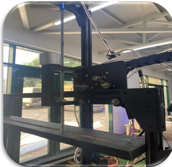
Figure 14 : Counterweight on Y-axis for balanced vertical movement.
