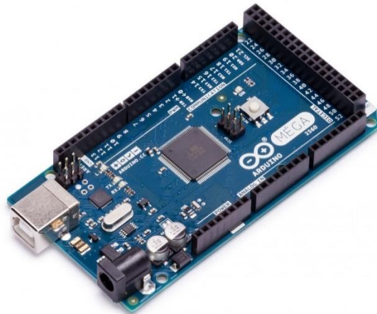
Figure 9 : Arduino Mega controlling the RootRise system.
