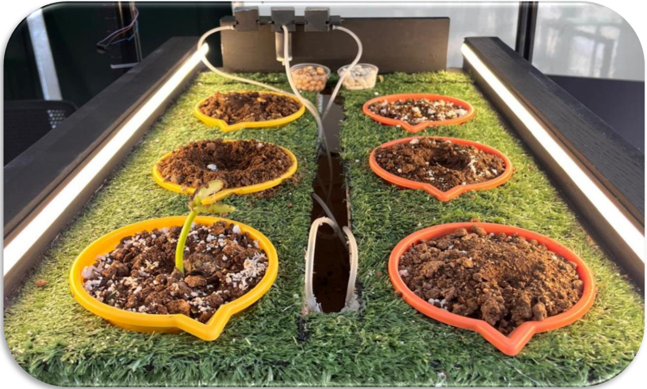
Figure 24 : Control the 4K linear lights manually or automatically via the LDR sensor.
