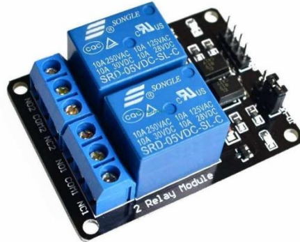
Figure 28 : Relays for safe and automated device control (2).
