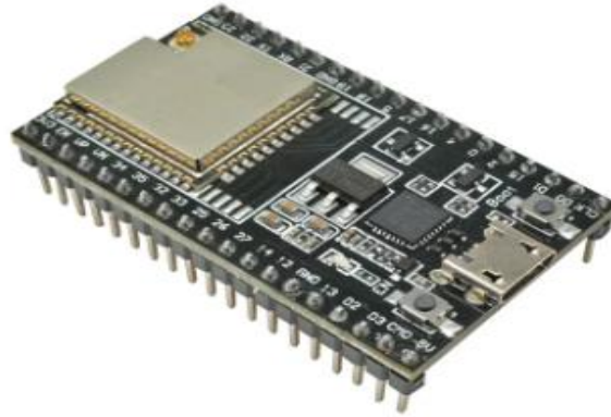
Figure 2 :ESP32-DevKitC ESP32-WROOM-32U Core Board
