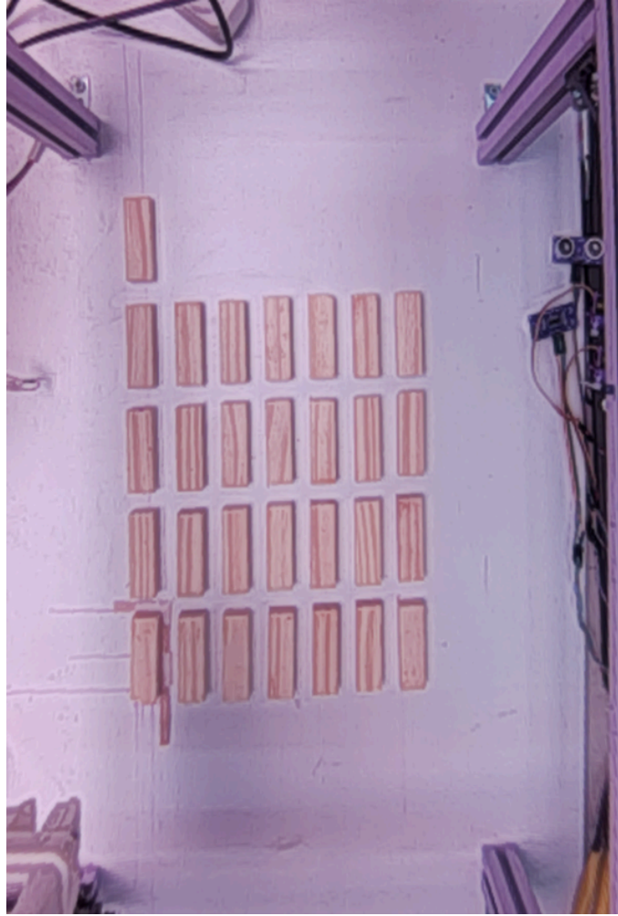
Figure 17: The vision reference board: 29 blocks on the vertical grid, the aluminium rails at the frame edges, and the holder's two wooden offcuts beside cell [0,0]. The magenta cast is the camera's uncorrected colour response.
