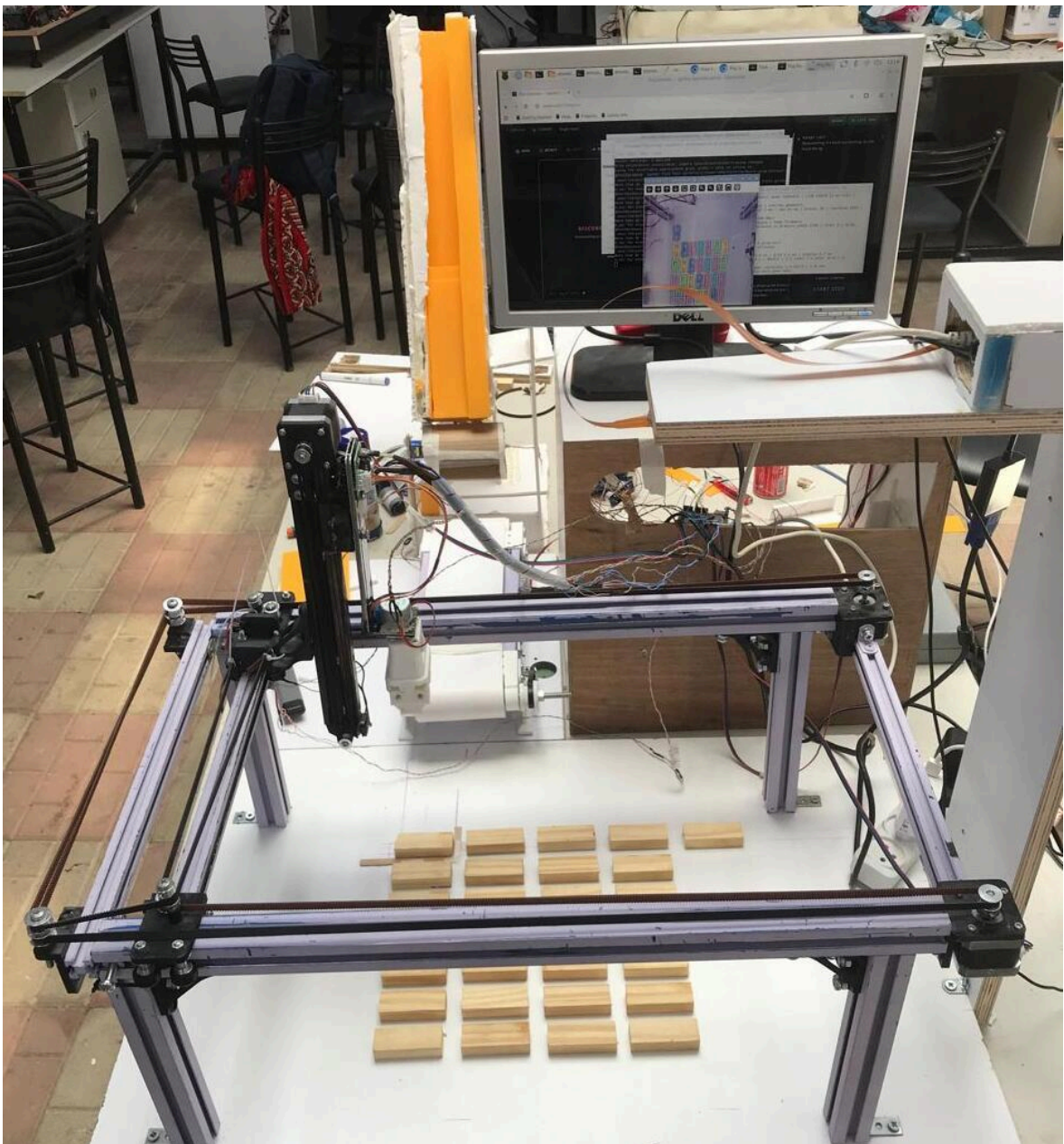
Figure 1: The completed rig: CoreXY gantry, Z axis and claw, feeder module on the left, and the overhead camera on its wooden support frame.
