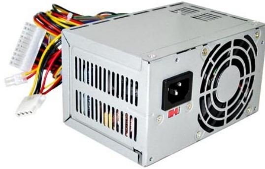
Figure 22: pc power supply
