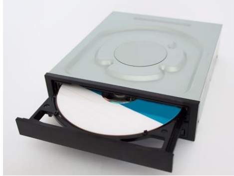
CDROM with DC motor for z axis
