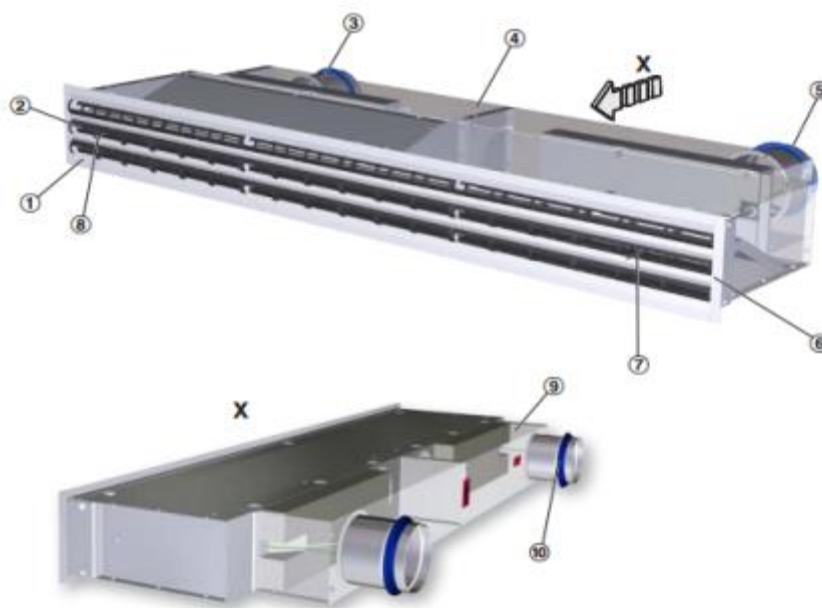
Figure 315: Slot diffuser unit (2).
