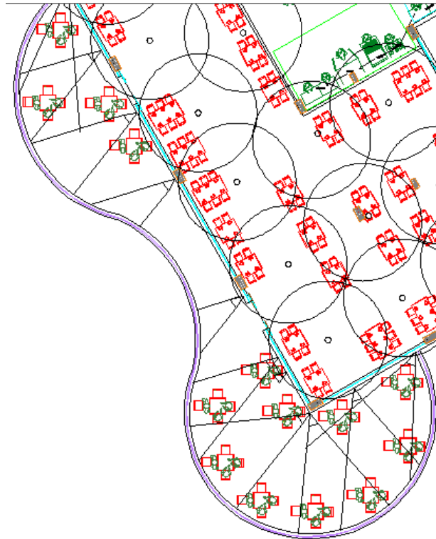
Figure 280: Wall mounted speaker distribution.
