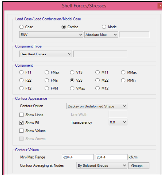
Figure 187: shear contour value - min and max range .
