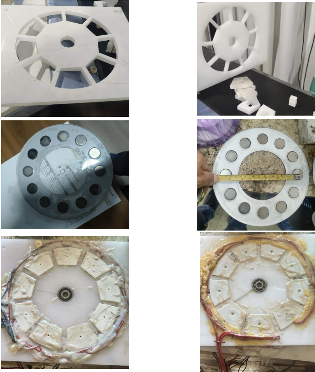
Figure 74: step-by-step construction of the axial flux stator and rotor components
