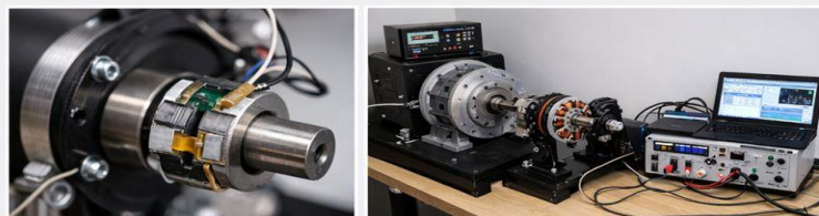
Figure 9.3: Embedded torque sensor with strain gauges
