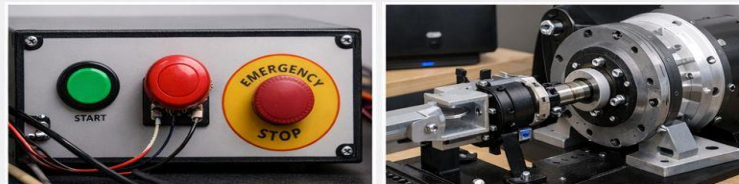
Figure 9.5: Control and Safety Panel with Emergency Stop
