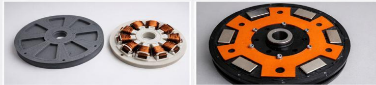
Figure 9.1: 3D-printed rotor and Stator assembly
