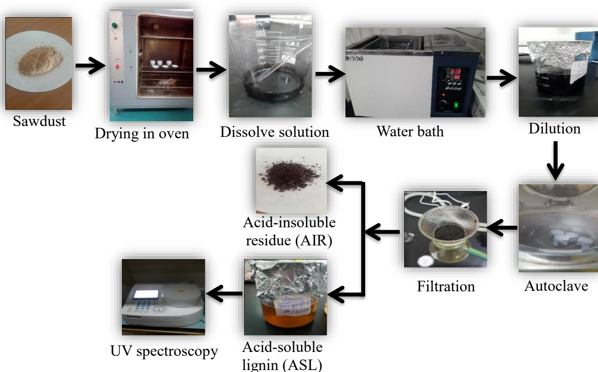
Figure 18: Procedure for lignin content measurements in sawdust and pulp.
