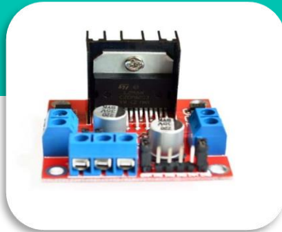
Dual H-Bridge Motor Drive
