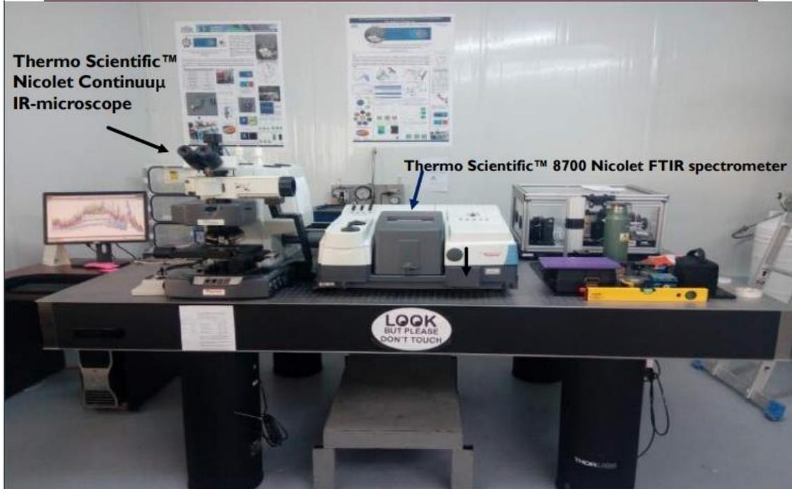
**Figure 2.7:** The end station of IR beamline at SESAME is equipped the 8700 Thermo Scientific© FTIR spectrometer coupled with the Thermo Scientific© Nicolet Continuum IR-microscope.
