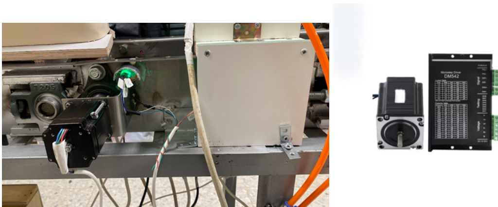
Figure 6.2.15: Advanced stepper motor Nema 23 and driver TB6600 for conveyor belt
