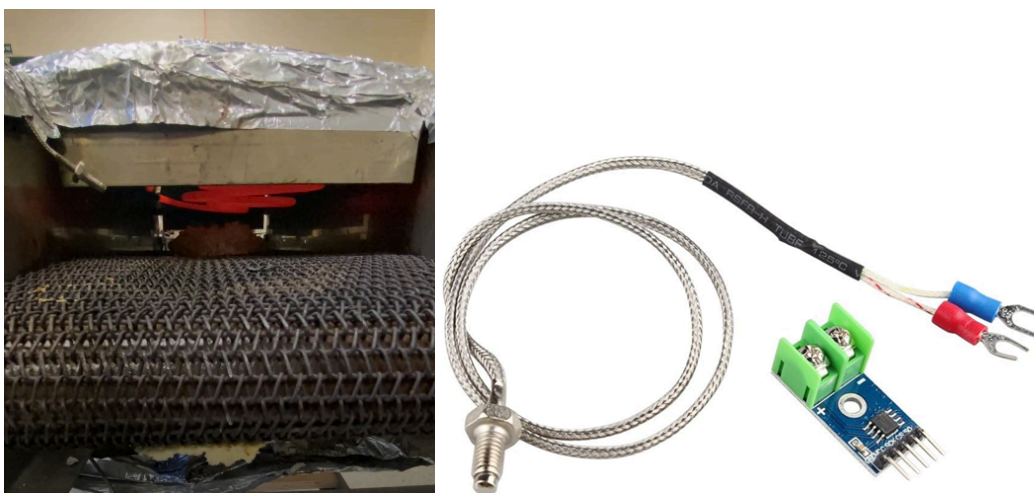
Figure 6.2.14.2: Thermocouple Temperature Sensor Module MAX6675
