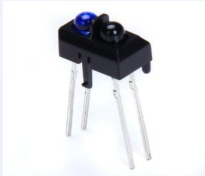
IR receiver transmitter (TCRT5000)
