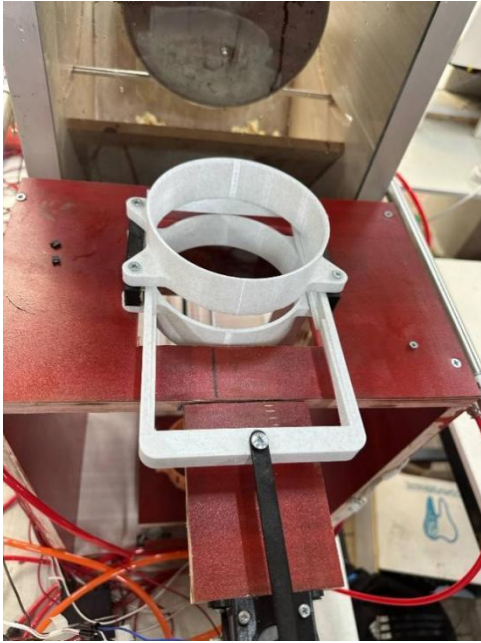
Fig. 4.2: Cup Dispenser Mechanism
