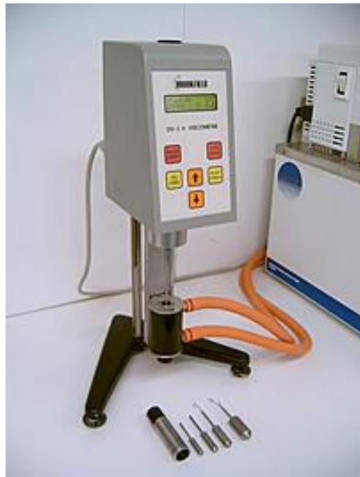
**Fig. (3.1)** A Brookfield Viscometer Model DV-I+ with UL adapter
