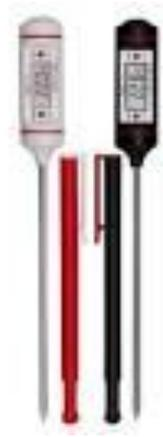
**Fig. (3.2)** Digital Prima Long Thermometer
