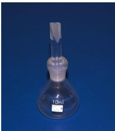
**Fig. (3.4)** Pycnometer
