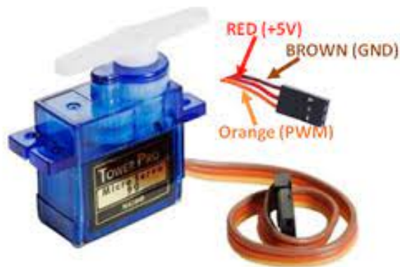
Figure 3: Servo Motor-SG90
