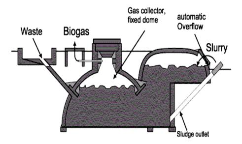
Figure 6 Fixed dome plant CAMARTEC design
