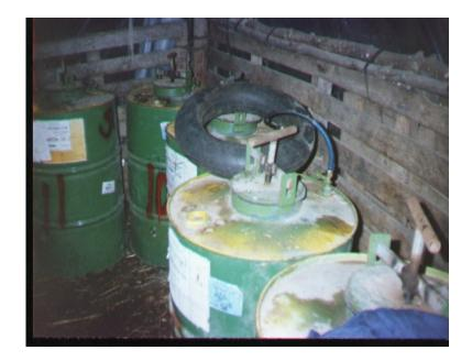
Photo 9 Withdrawing biogas from barrel digester into tube.
