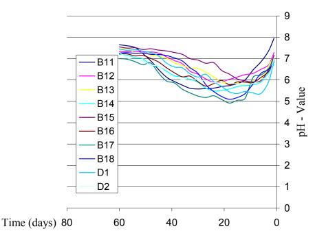
Figure 16 pH changes with time for samples from B11 to B18 and D1, D2
