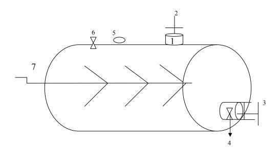
Figure 11 Schematic diagram of 1.5m<sup>3</sup> digester with stirrer:- 1- Inlet open,
