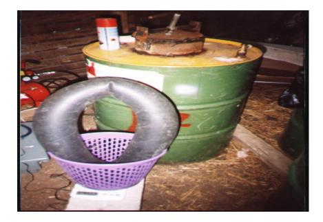
Photo 11 Weighting biogas by digital balance.
