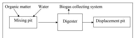
Figure 2 Schematic of the basic components for the biogas plant.
