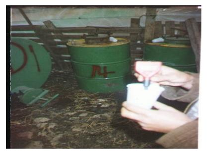
Photo 8 Measuring slurry pH.
