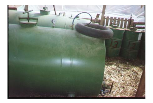
Photo 10 Withdrawing biogas from large digester into tube
