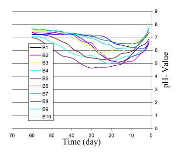
Figure 15 pH changes with time for samples from B1 to B10
