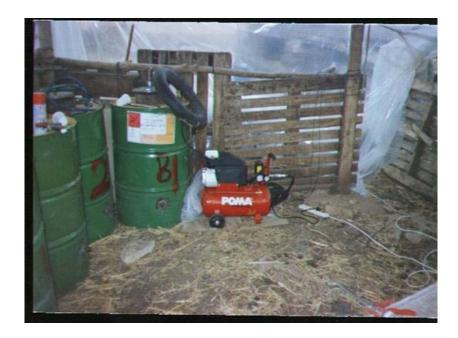
Photo 12 Withdrawing biogas from tube by the compressor.
