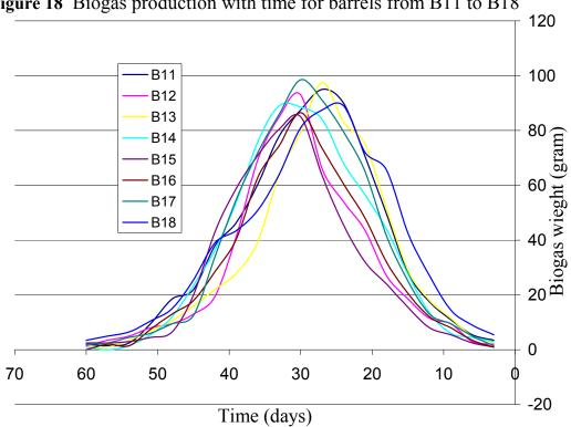
Figure 18 Biogas production with time for barrels from B11 to B18
