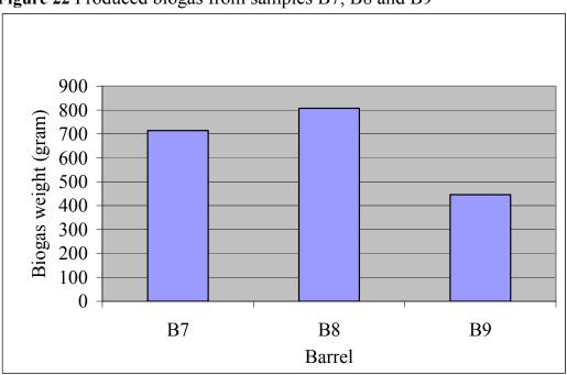
Figure 22 Produced biogas from samples B7, B8 and B9
