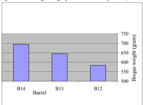
Figure 23 Total biogas weight produced from samples B12, B13 and B14
