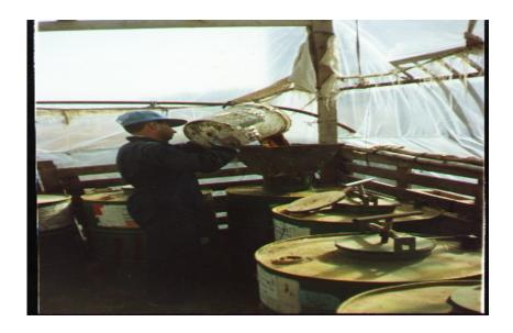
Photo 6 Introducing sample into the digester
