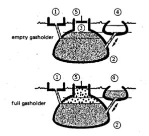
Figure 4 Basic function of a fixed-dome biogas plant, 1- Mixing pit, 2- Digester, 3- Gasholder, 4- Displacement pit, 5- Gas pipe
