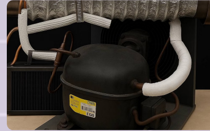
Copper pipes with circulating refrigerant (compressor + radiator).
