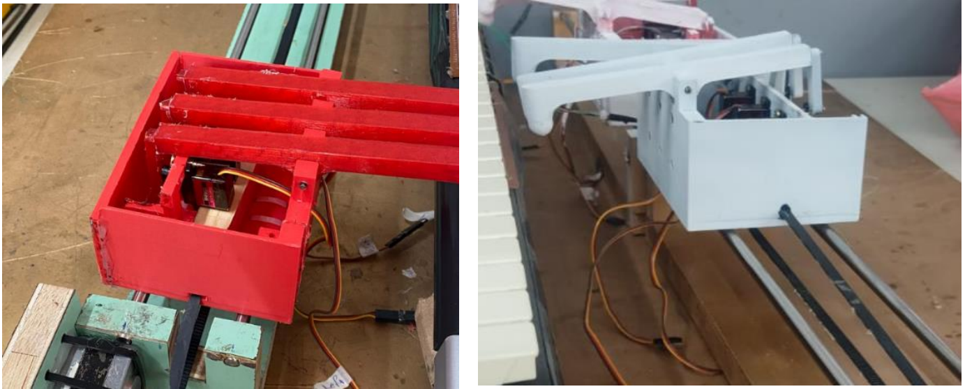
Figure 3.11: Finger controlled using MG90S Servos.
