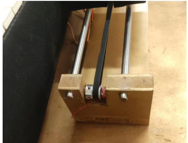
Figure 3.9: Two parallel 8mm stainless steel rails.
