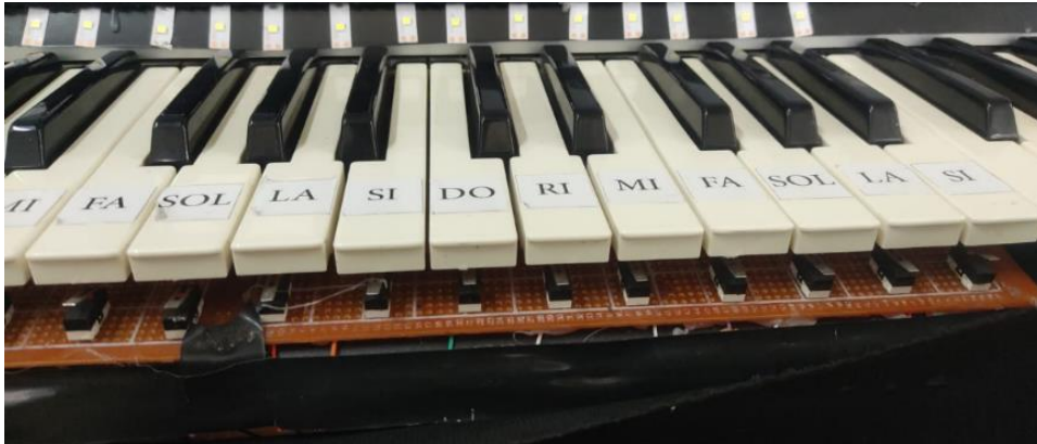
Figure 3.4: Mini switches positioned under the 14 keys.
