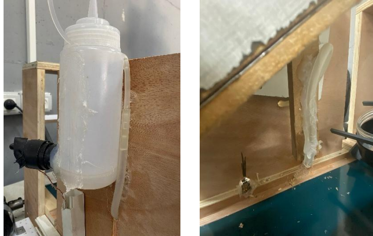
Figure 6.2.15: Oil Dispensing Pump
