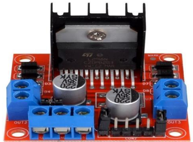
Figure 33-3-6-1 DC motor Driver
