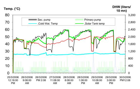
Fig.6-a: Temperature distribution in the SWH, solar radiation, and water flow consumption and primary pump work time from 25-30 March 2006.
