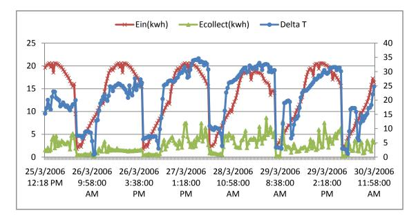
Fig.8-a: Input solar energy and collector output energy with the coressponding temperature difference. (25-30) May/2006
