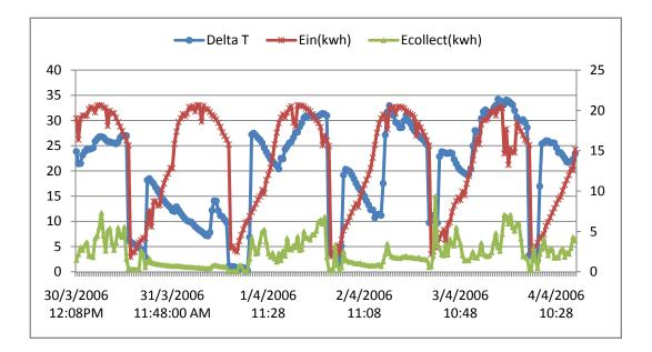
Fig.8b: Input solar energy and collector output energy with the coressponding temperature difference.
