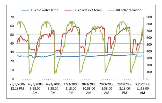
Fig.6-b: Solar tank and collector exit temperatures in the SWH and solar radiation from 25-30 March 2006.
