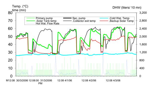
Fig.7-a: Temperature distribution in the SWH, solar radiation, and water flow consumption and primary pump work time from 30March to 3 April 2006.
