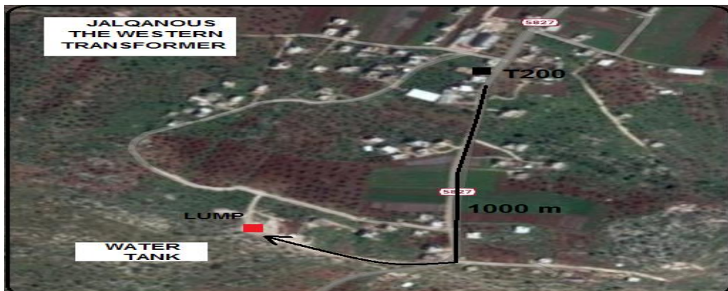
Figure (A.2.43) : The large loads on transformer(T200) in Jalqamous village network in reality
