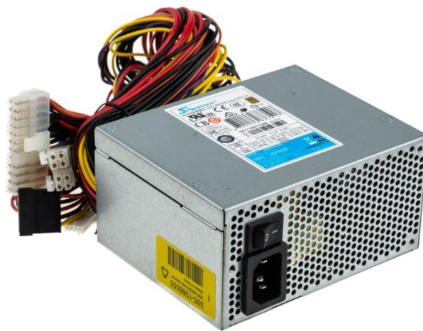
Figure 22 PC Power Supply
