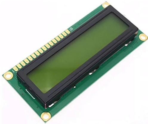
Figure 4.13: 16x2 LCD Screen
