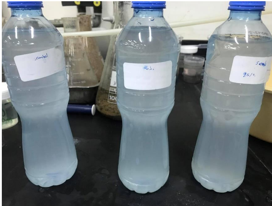
Figure A 7: Coagulation Experiment of Treated Moringa Using Plastic Bottles.
