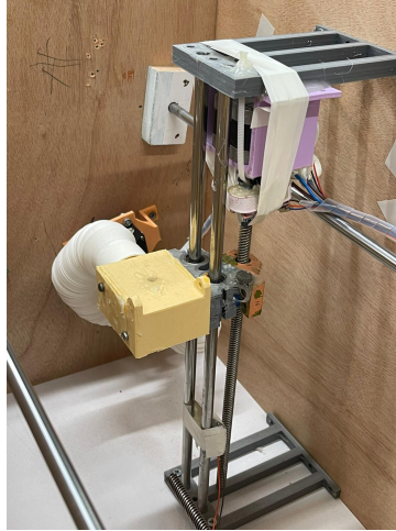
Figure 3.15: Vertical glove pickup mechanism including the stepper motor, linear motion assembly, shaft coupler, and threaded rod.
