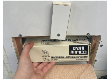
Figure 3.12: Side access port used for inserting and refilling glove packets while maintaining an airtight enclosure.
