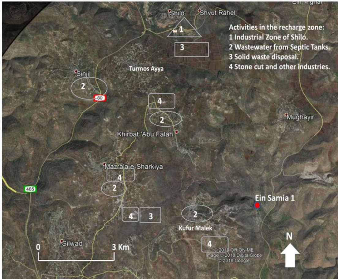
Figure (2.5): Aerial Map of the Recharge Area, Identifying the Anthropogenic and Industrial Activities which Affect the Appearance of Pollutants in the Spring (Dr Saed Khayat, 2018).
