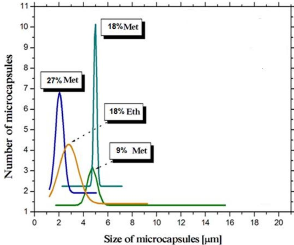
**Figure 3. 4 (b):** The size distribution of PLG microcapsules prepared with different concentration of methanol and ethanol.
