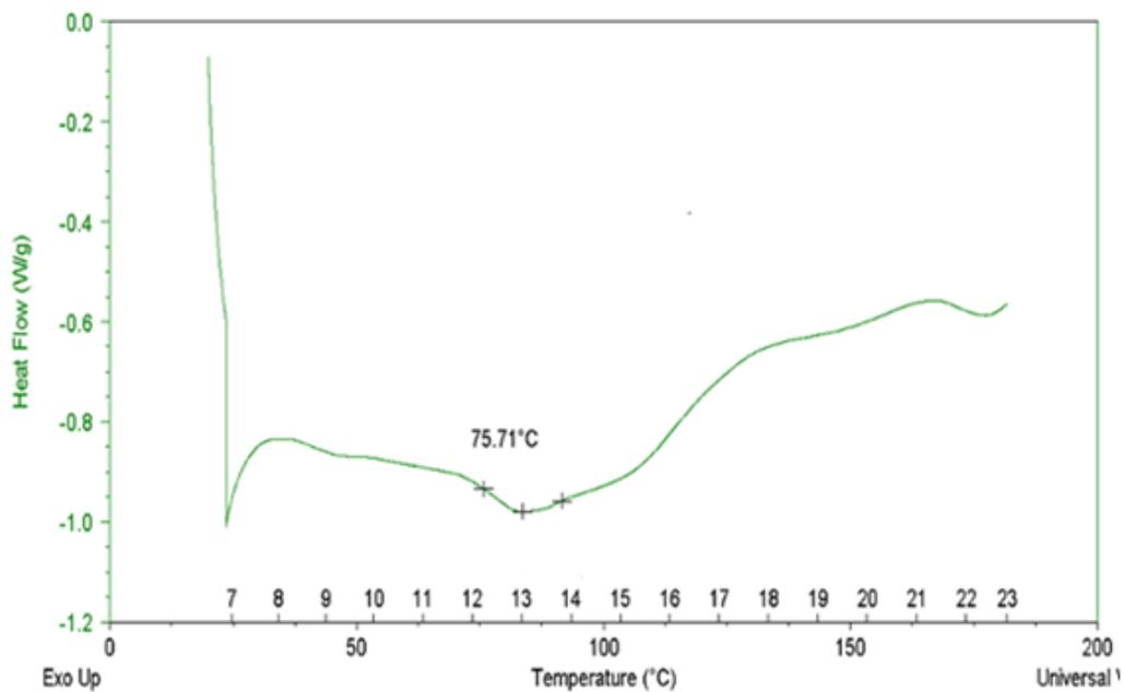
**Figure 3.6.** DSC result for PLG microcapsules prepared with 10% SDS solution.
