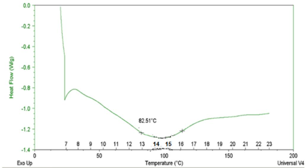
**Figure 3.10:** DSC result for PLG microcapsules prepared with 18% ethanol.
