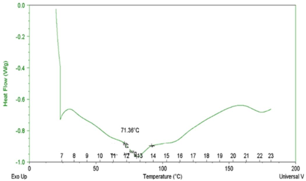
**Figure 3.7.** DSC result for PLG microcapsules prepared with 2% SDS solution.
