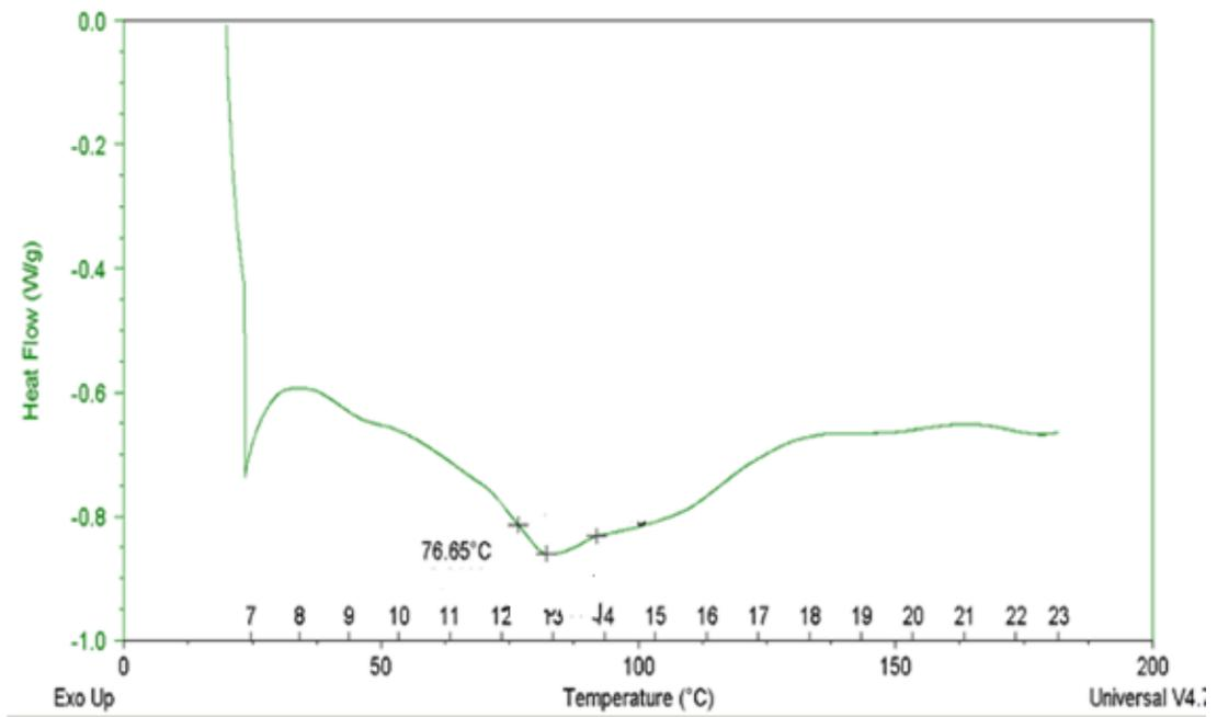
**Figure 3.9:** DSC result for PLG microcapsules prepared with 27% methanol.
