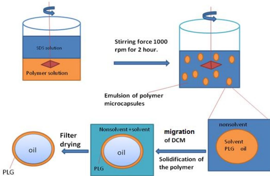
**Figure 2.1:** Preparation of PLG Microcapsules
