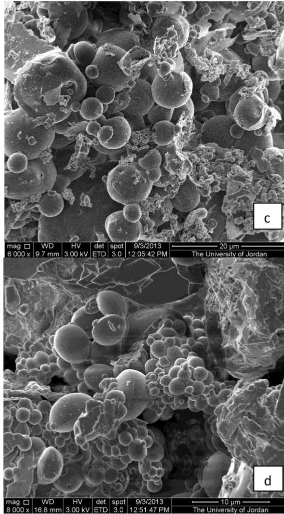
**Figure 3.5:** SEM micrographs of prepared microcapsules with a) 10% SDS, b) 5% SDS, c) 18% methanol, d) 18% ethanol.
