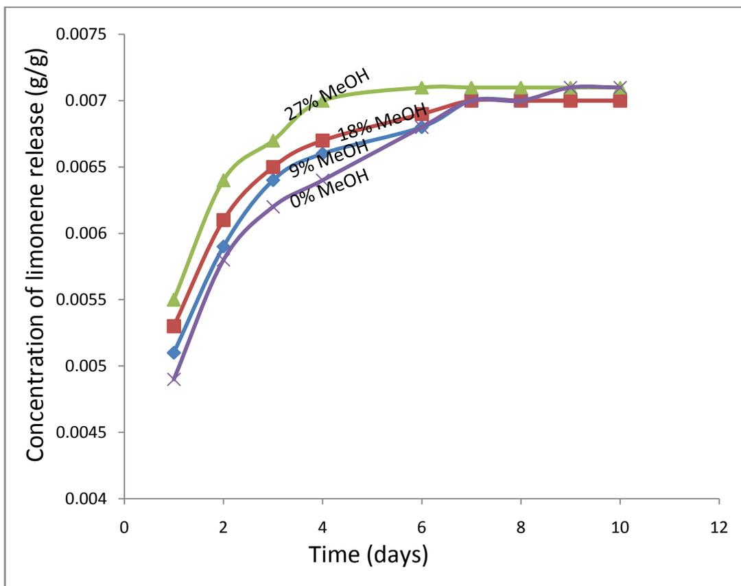
**Figure 3.13:** Limonene release from PLG microcapsules prepared with different amount of methanol solutions.
