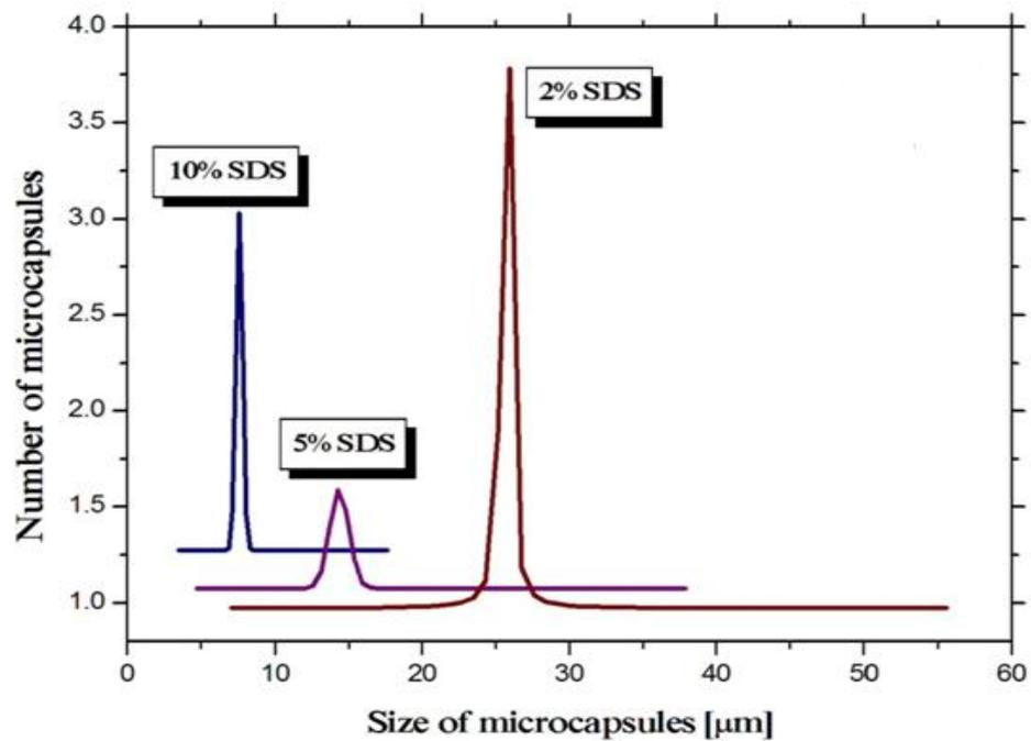
**Figure 3.2:** (b): The size distribution of PLG microcapsules prepared with different concentration of SDS solution.
