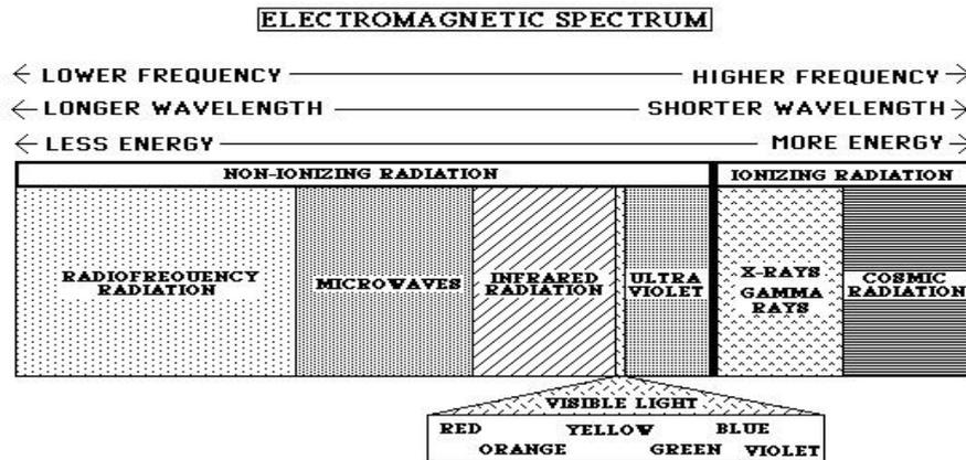
Fig.1: the electromagnetic spectrum showing the two types of electromagnetic radiation.
