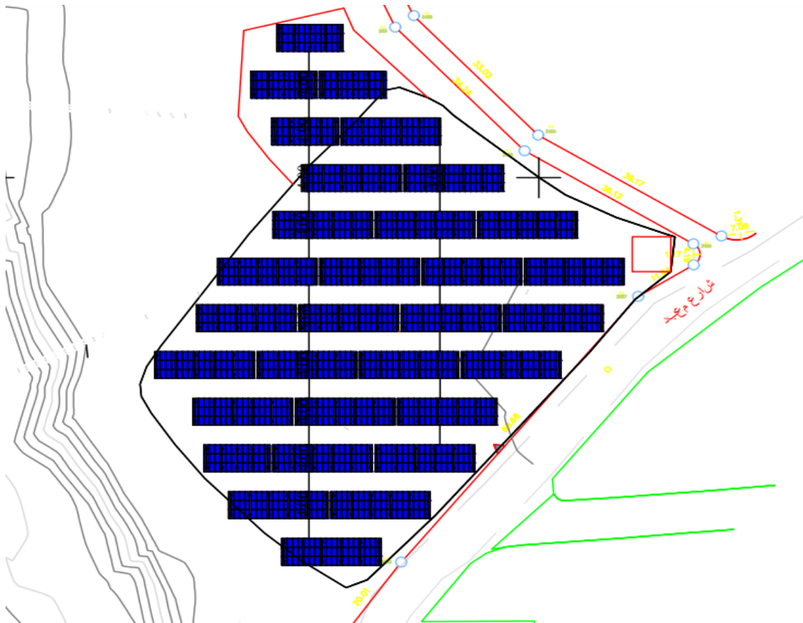
Figure (4.3): PV layout for 0.5 MWp system
