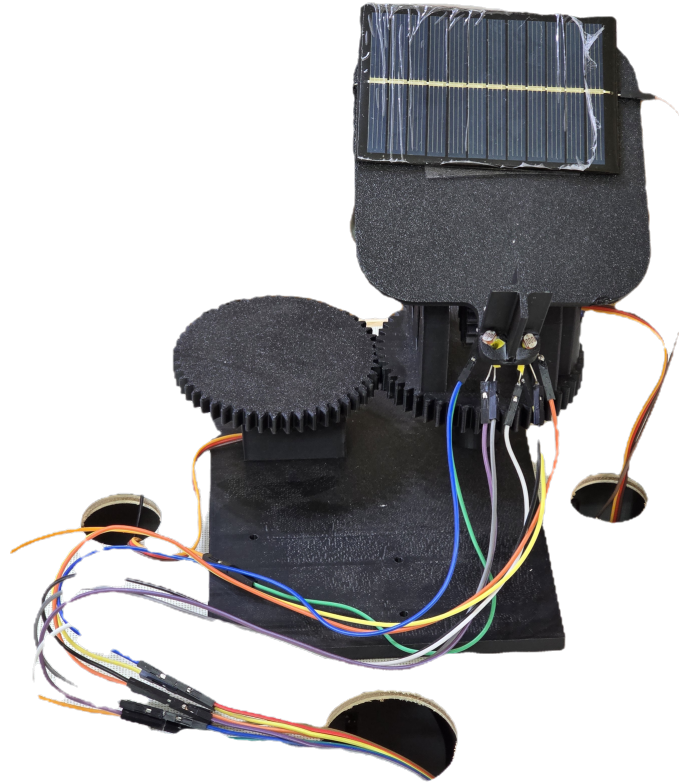
Figure 4.18: Fully assembled prototype front view showing solar panel, LDRs, and wiring
