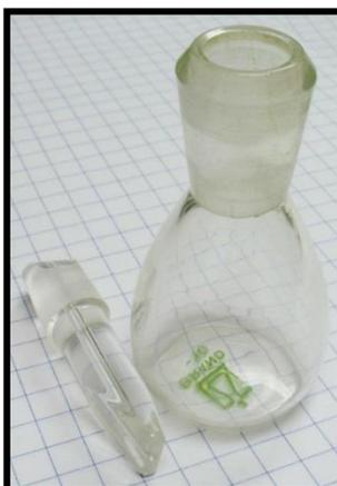
**Fig. (3.4):** Pycnometer of 10ml for density measurement.
