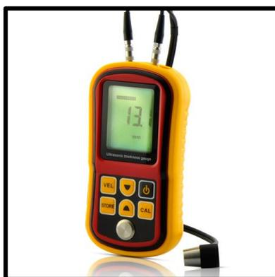
**Fig. (3.6):** Ultrasonic thickness gauge for sound velocity measurements.
